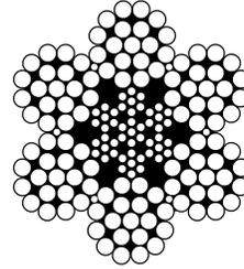
This class is most widely used and is found in its many variations throughout nearly all industries. With its combination of flexibility and wear resistance, rope in this class can be suited to the specific needs of diverse kinds of machinery and equipment. The designation of 6 x 19 is only nominal as the number of wires per strand ranges from 15 to 26.
