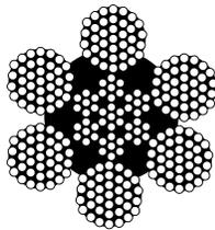
The 6 x 37 class of wire rope is characterized by the relatively large number of wires used in each strand. Ropes of this class are among the most flexible available, but their resistance to abrasion is less than the 6 x 19 class. The designation of 6 x 37 is only nominal as the number of wires per strand ranges from 27 to 49.
