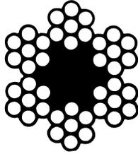
This construction is used where ropes are dragged over the ground or over rollers and resistance to wear abrasion are important factors. The wires are quite large and will stand a great deal of wear. The 6 x 7 is a stiff rope and needs sheaves and drums of large sizes. It will not stand bending stresses, as well as, ropes with a large number of wires.
