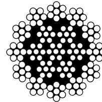
The 19 x 7 rotation resistant rope consists of an inner layer of 6 strands of 7 wires each, made left lang lay over a strand core, and an outer layer of 12 strands, each of 7 wires, made in right regular lay. It is this combination of opposing lays which enables the rope to resist the tendency to rotate when in service.
